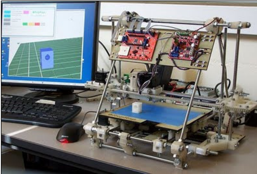
Figure 15. RepRap rapid self-replicating machine
